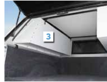
Toolboxes are securely fastened to roof framework
